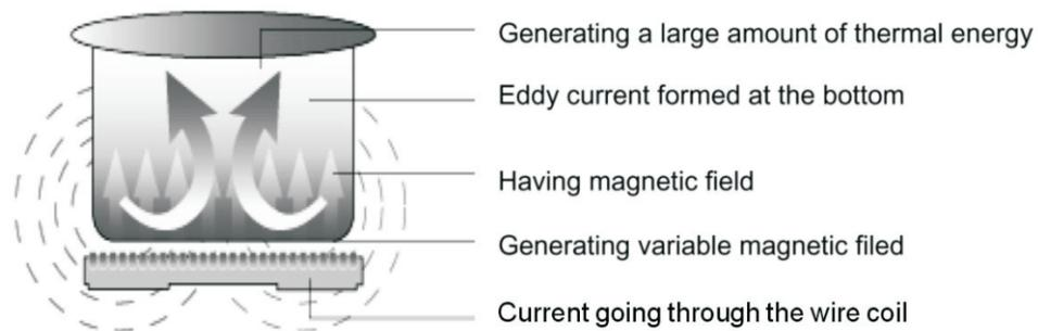
The induction cooker is mainly based on the principle of electromagnetic induction technology. Current generates variable magnetic field after running through the wire coil. Eddy current is generated at the bottom when the magnetic field induces the cooker plate. A large amount of thermal energy produced can heat the bottom quickly, thus heating up the food very fast, with thermal efficiency up to 94.36%.
